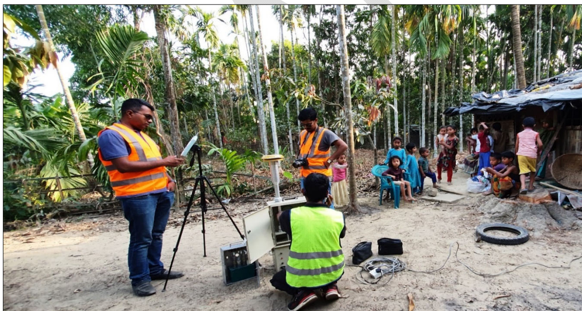
Figure_Apx 82: Photograph demonstrating field level noise EIA technique.
