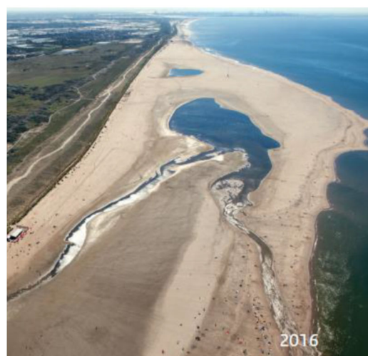
Figure 4.17: Nature based sand engine in The Netherlands
